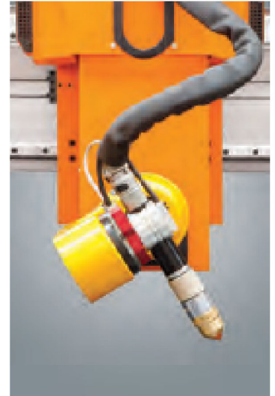
Can move totally \pm 50 and 600 degrees at B axis.
