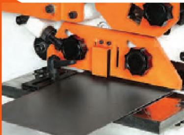
Flat sheet metal cutting station
