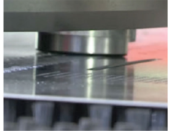
Smooth cutting of sheet metal in requested shape with punch tools up to 88.9 mm In diameter (S)
